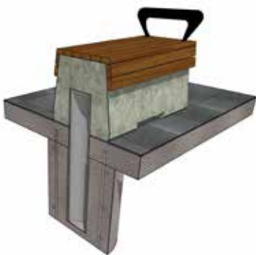
Typical steel reinforced fixing pin installation
