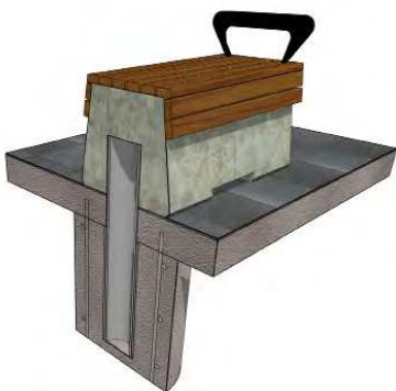
Typical steel reinforced fixing pin installation
